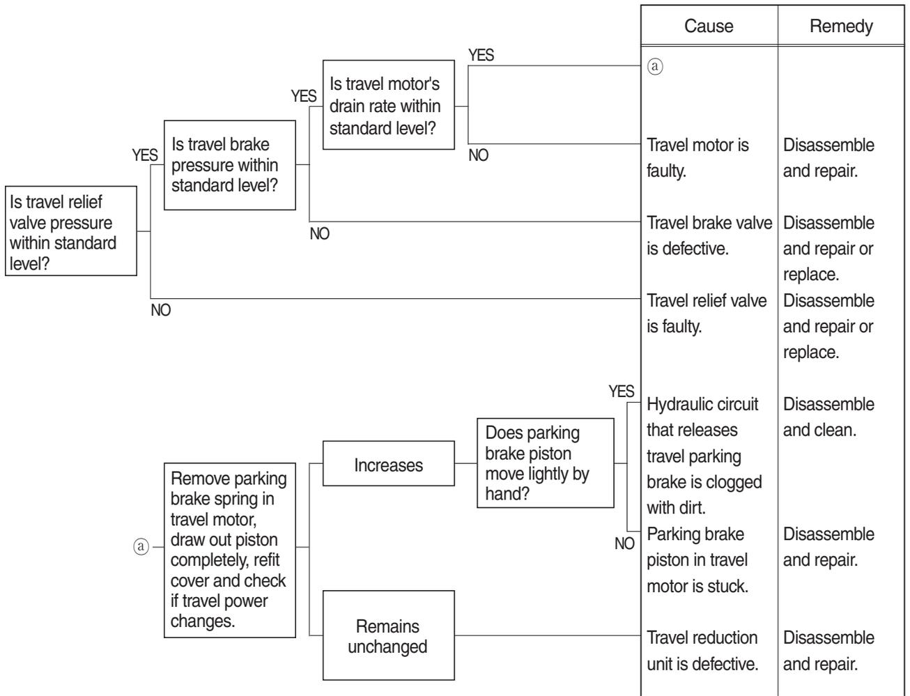
**6) MACHINE RUNS RECKLESSLY ON A SLOPE**
